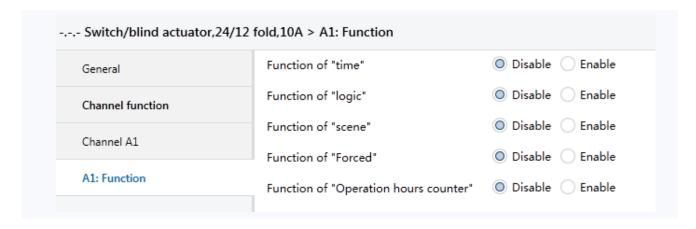
Fig. 4.5 the special function enable window " $X_{1,2}$ : Function"
