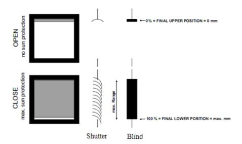
The functions described for the "Shutter" operating mode also apply to the "Blind" operating mode (with the exception of the slat adjustment function).
