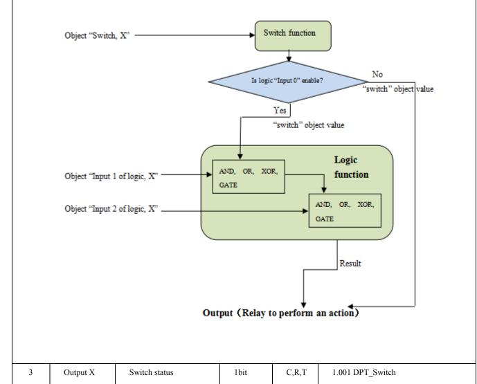
This object indicates the contact status (details will be defined by parameter "Object value of switch status:" in "Channel  $X_{1,2}$ : Switch").
