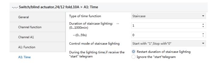
Fig. 4.8 parameter window "X<sub>1,2</sub>: Time-staircase"
