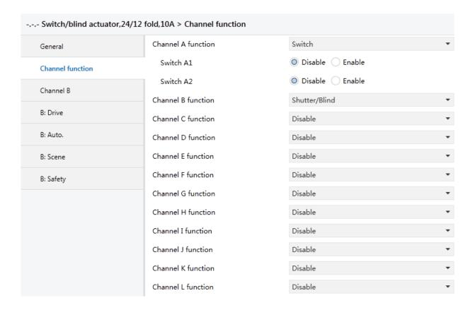
Fig. 4.2 Parameter Window"Channel function"
